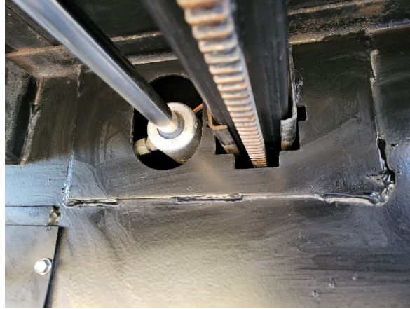
Figure 42. Frame view of the early-model Paradigm trailers with gear pack inside the frame.
