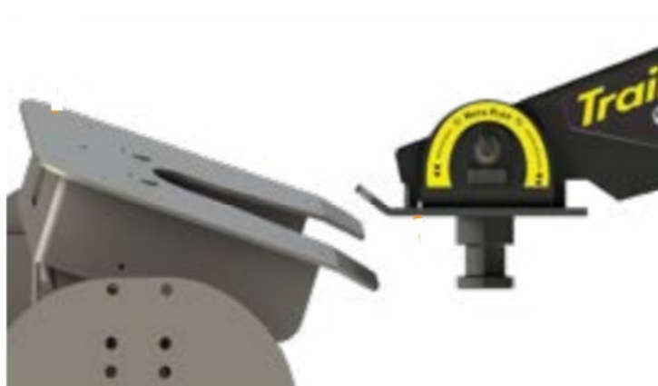
Figure 21. Appropriate vertical position to assure safe kingpin capture: flat pin box plate rides up the hitch ramp.
