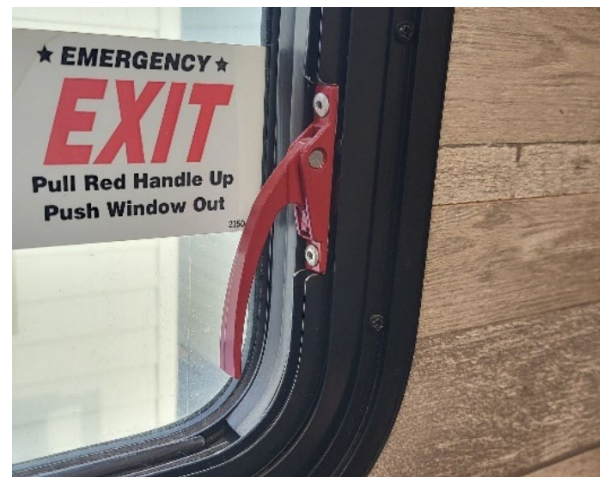
Figure 28. Pull-Lever style latch on an emergency exit. Pull the lever out, away from base, to disengage latch. Push window out.
