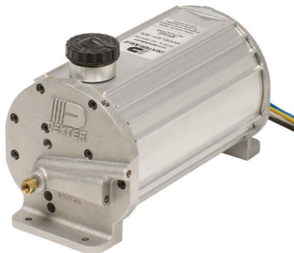
Figure 6. Dexter Brake Actuator.
