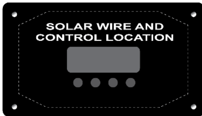
Figure 92. Label used to indicate pre-wired location of solar control mounting on early model Alliance trailers.
