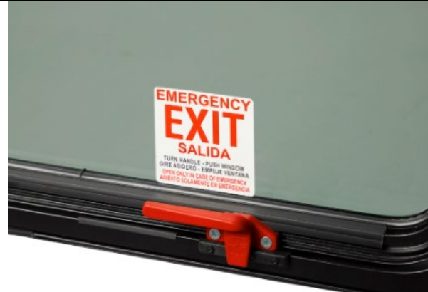
Figure 27. Rotation-Lever style latch on an emergency exit. Rotate the handle up into the window area to disengage the latch. Push window out.
