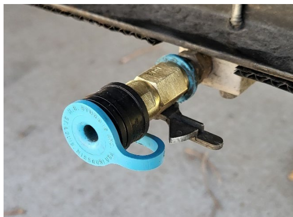
Figure 35. External propane quick connect, with flow lever in the "off" position.
