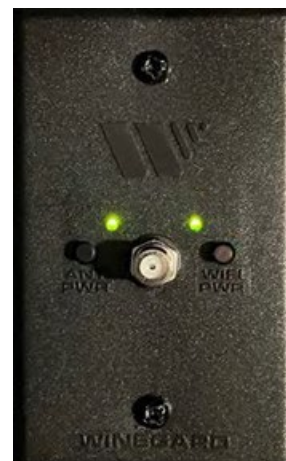
Figure 119. Winegard booster switch, with booster and Wifi enabled.
