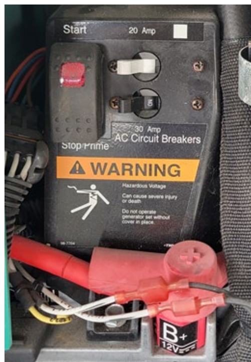
Figure 117. On-board controls for the Onan 5500 generator. The start/stop button and integrated fault light are on the left, and circuit breakers are on the right.
