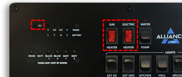
Figure 142. The water heater power switches on the main Monitor Panel. The FLT light is highlighted on the left. These are also shown in Figure 121A and D.
