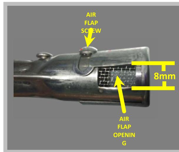
Verify air flap screw is tight and opening is 8mm (5/16"). If not, adjust air flap opening to 8mm and tighten.
