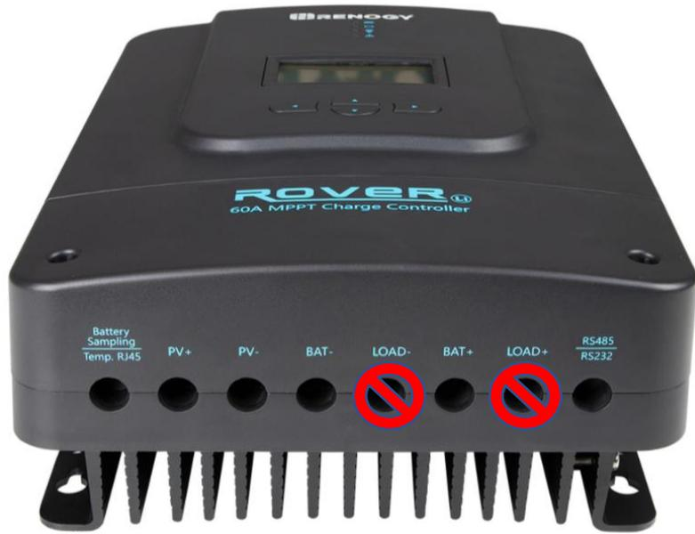
Check voltage on display screen to verify if wiring is correct
