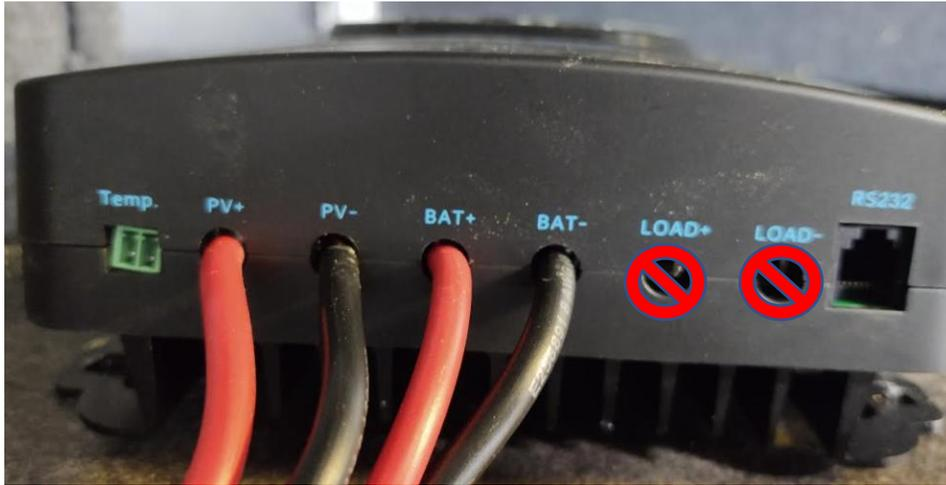
Check voltage on display screen to verify if wiring is correct
