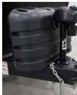
Protective cover with easy access hatches for valve and shutoff.
